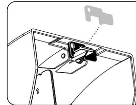
Unlock key is stored with spring clip under top of bucket
